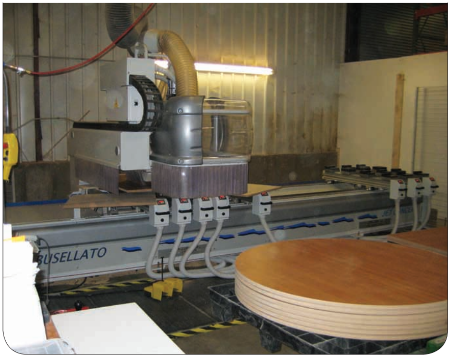
Bruewer Woodwork's demand is established first, and then equipment such as this Busellato Jet machining center is implemented to meet that demand.
